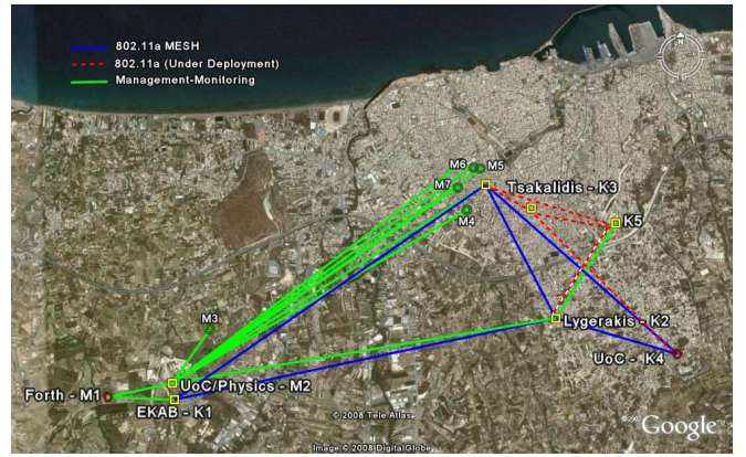
Fig. 4. Experimental metropolitan wireless multi-radio mesh network in Heraklion. The five links considered in the experiments involve the four nodes K1-4. Nodes M1-8 are used solely for management and monitoring.
